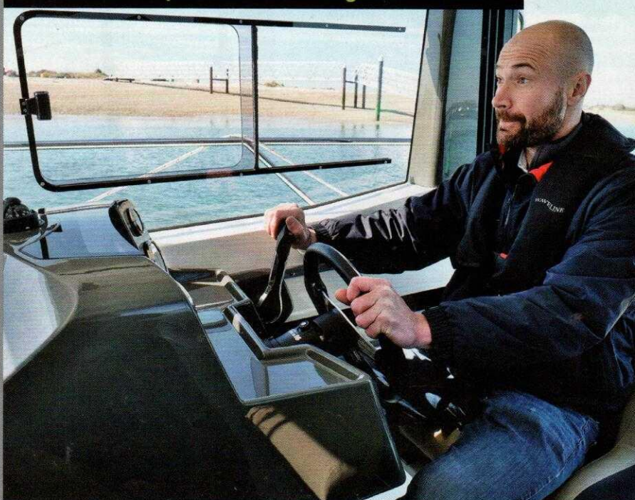
Enclosed helm position has sliding side screens
